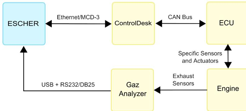
Figure 6: Experimental Set-Up for the Tests on a Real Engine
