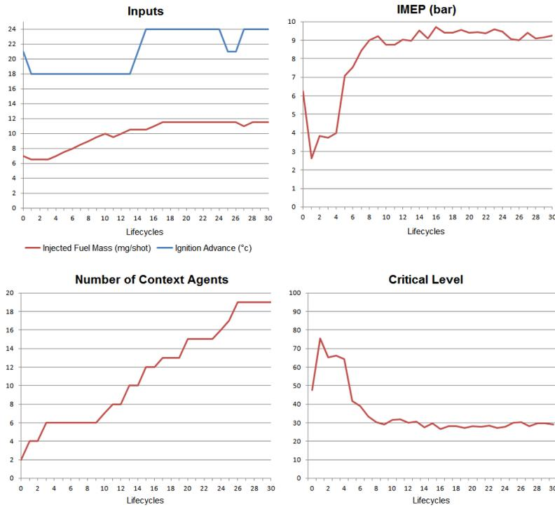
Figure 7: IMEP Optimization while Controlling Two Parameters
