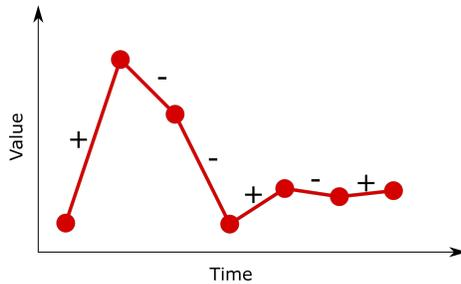
Figure 3: Typical Convergence of an Adaptive Value Tracker
